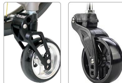
The Shockwave XIX has suspension options for the front castors.
