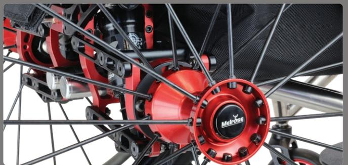
The Melrose Shockwave XIX is a fixed position wheelchair designed and built to provide a comfortable ride by reducing jarring and vibration while negotiating tiled surfaces, cobblestones or going up and down curbs and steps. We have achieved this by building a parallel 4-link suspension component for the rear wheels, this part is adjustable for preload (weight) damping and
